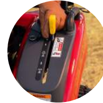
1. PTO lever for mid- and rear rpm
